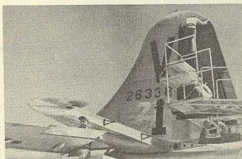
Removing tail surfaces from the B-29 going through an overhaul in the maintenance division.
