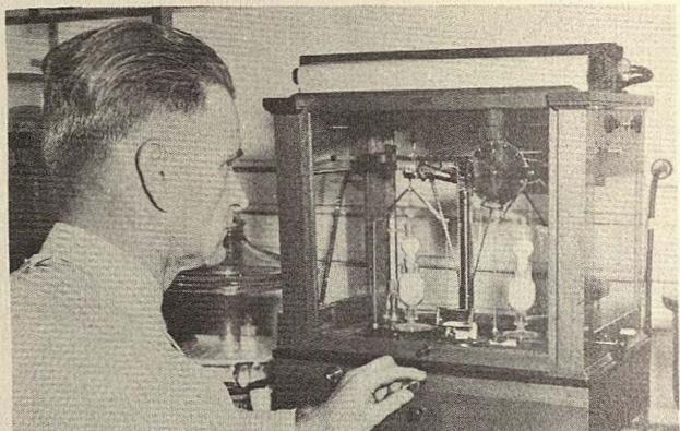
Test samples are weighed out in the chemical master control laboratories of the Maintenance shops.
