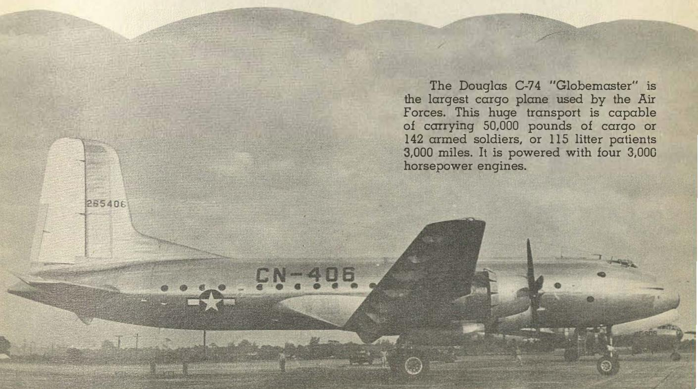
The Douglas C-74 "Globemaster" is the largest cargo plane used by the Air Forces. This huge transport is capable of carrying 50,000 pounds of cargo or 142 armed soldiers, or 115 litter patients 3,000 miles. It is powered with four 3,000 horsepower engines.
