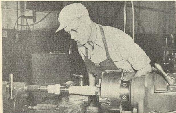
Precision is the byword in such work as rolling a flange on the impeller drive shaft of an R-2000.
