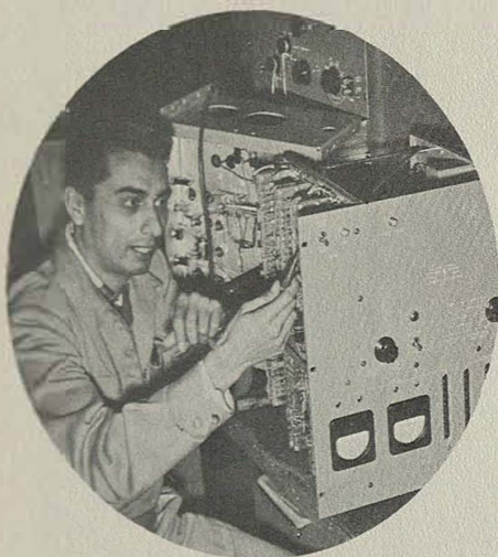
Radio model "SCR-522" air borne model shows transmitter and receiver undergoing final check, this model operates on very high frequency.
