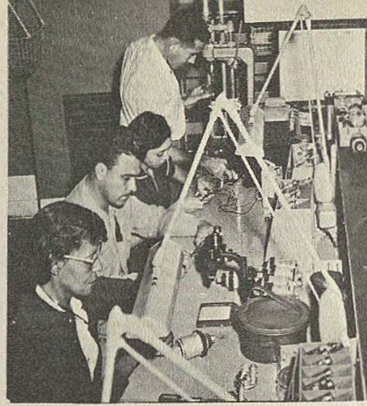
▲ Bldg. 326, calibrating autosyn transmitters.
