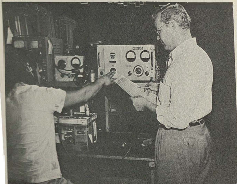
Radio model "SCR-522" air borne model shows transmitter and receiver undergoing final check, this model operates on very high frequency.
