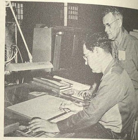
▲ Bldg. 326, calibrating autosyn transmitters.
