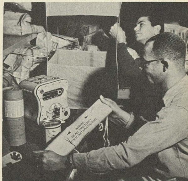
Making up an emergency kit to go with the "Gibson Girl" radio. In the rear is the box kite to carry the antenna, the tall can contains chemical to make hydrogen gas and the small can has the balloon to send the an-
