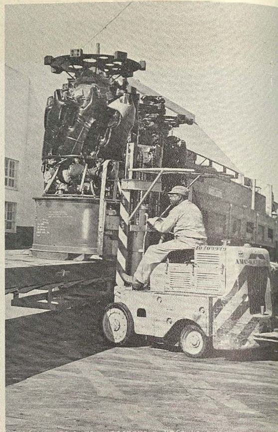
Finished B-36 engine is loaded on truck after being tested in the Engine Test Branch
