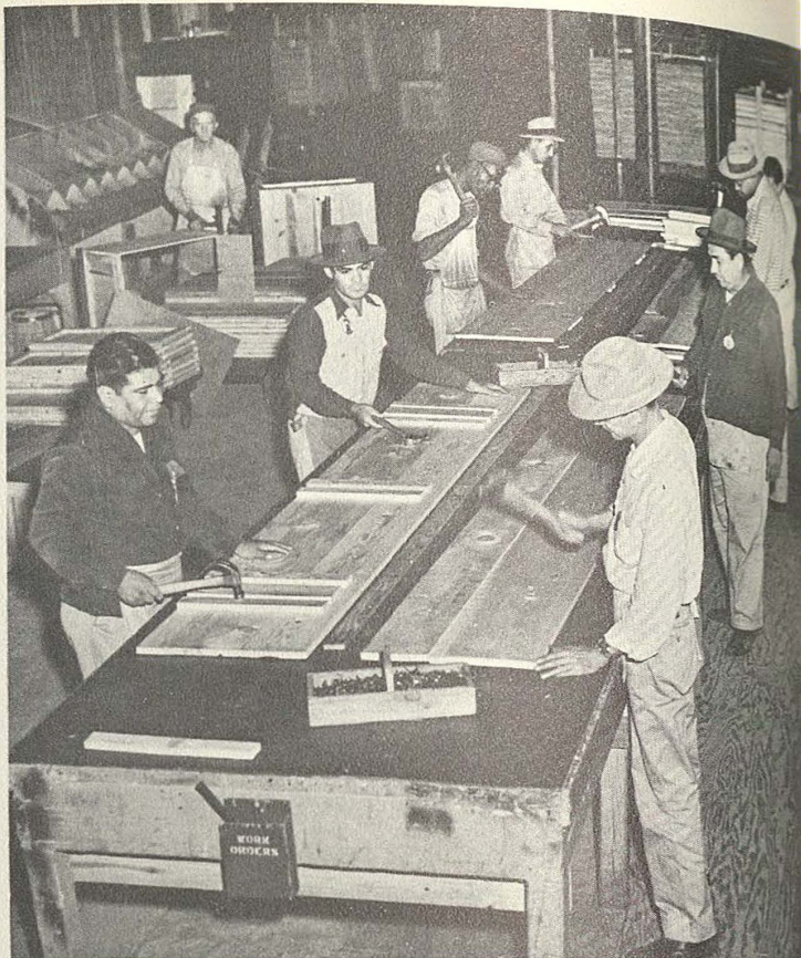
Speedy nailing crates together ready to be quickly assembled by sections.
