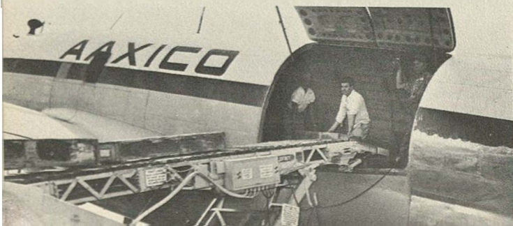
Conveyors extend right into cargo carriers.
